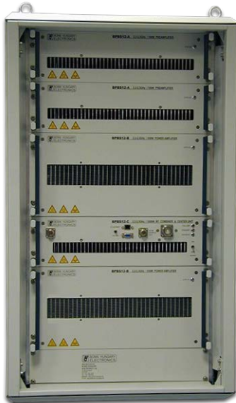
Figure 11. Redundant S band amplifier system with 1 kW output power
